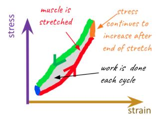
4. The graph shows the work loop of insect flight muscle. The graph shows how stress not only increases as strain increases, but continues to increase even after
